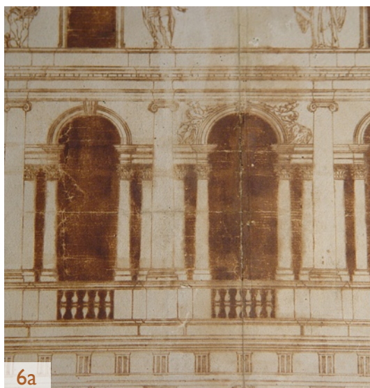
6.a-b Vincenzo Scamozzi, Elevation of the front of "Palazzo Nuovo" of Bergamo, Bergamo. Visible and IR detail. Reflectography helps to visualise damages and retouches, while original ink disappears in NIR short bands
